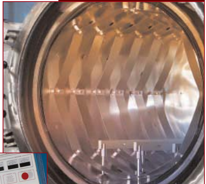
Above: The Performer Series 24" W x 24" H x 36"D all Molybdenum Hot Zone
