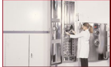
Evaporator with five planets and a magazine type load lock for increased productivity
