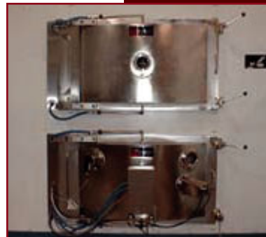
Side sputter system with etch and heat in the load lock
