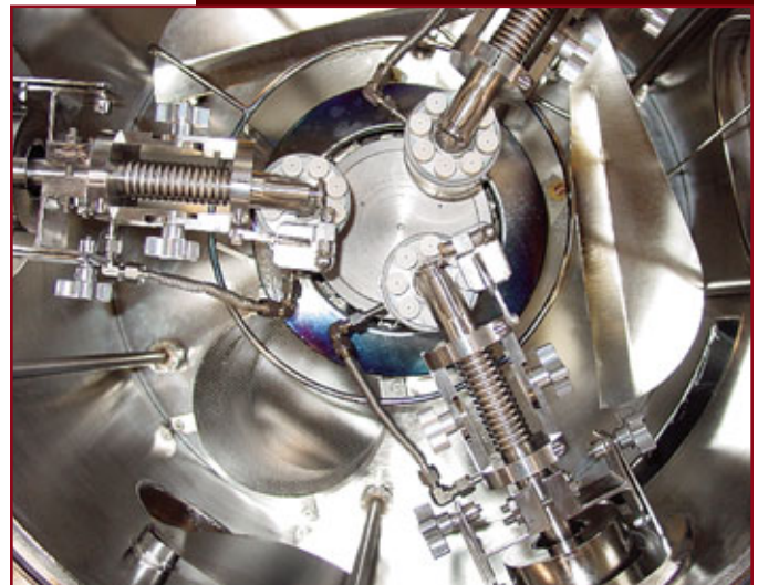
X, Y, Z adjustable Round Cathodes Capable of sputtering up, down or sideways
